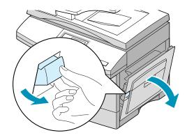
4 Carefully remove the misfed paper in the direction shown.
